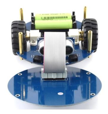
6. Assemble (1) and (2) with screws. Insert micro:bit board to AlphaBot2, set LED toward outside.
