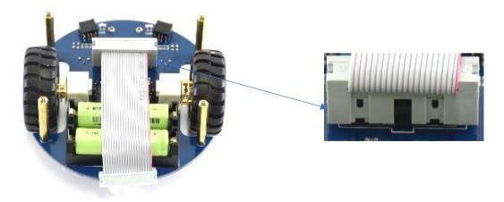
4. Insert (4) Ultrasonic sensor to 4PIN connector of (2) AlphaBot2-Basic
