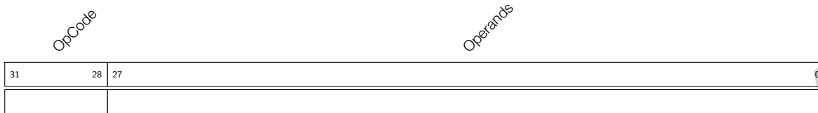
Figure 1-6. ULP-FSM Instruction Format
