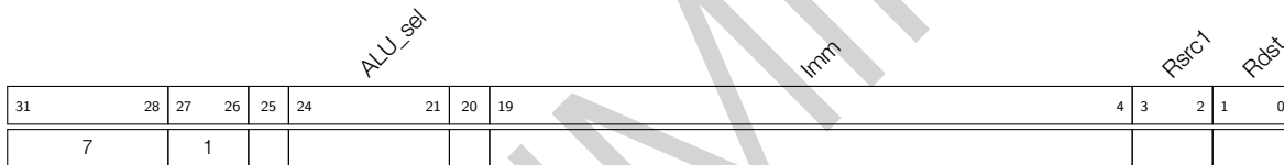
Figure 1-8. Instruction Type — ALU for Operations with Immediate Value
