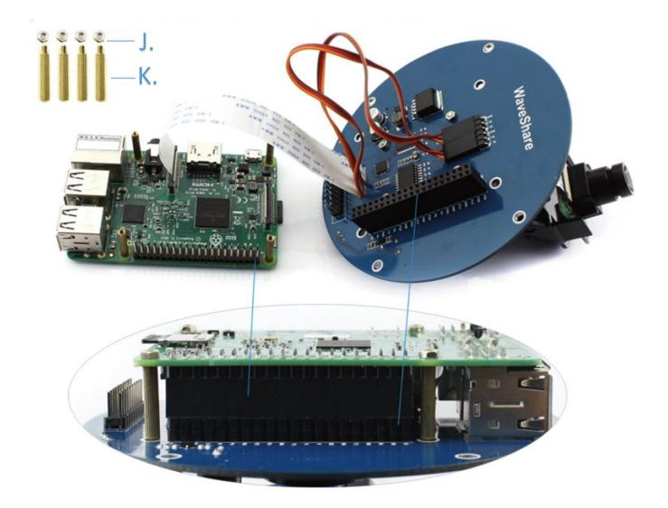
Plug the FC-20P cable to both the AlphaBot2-Pi (adapter board) and AlphaBot2-Base (base chassis). Note: the connector of the cable must be plugged following the marks on the PCB. Please make sure
