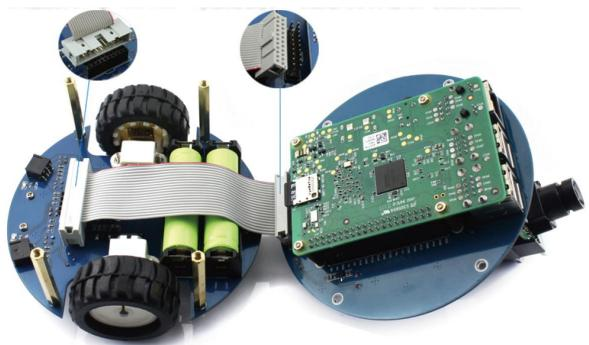
Fix your Pi to the AlphaBot2-Pi (adapter board) with the screws (I). Fix the AlphaBot2-Pi (adapter board) to the AlphaBot2-Base (base chassis) with the screws (F).
