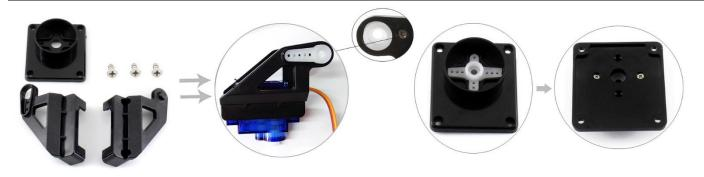
Insert the steering gear describe above to cross-shape rocket arm (b) in the stand (d) and fix the installation with a screw (1). Fix another steering gear into the stand (e), and fix it with two screws (7). Install the stand (e) and steering gear to the stands (f) and (g), and fix them with the screw (1).
