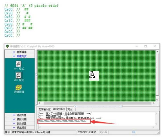
The font data can be got from the font modulo software which extracts the modulo of the font horizontally and vertically, and displays each pixel with an array. For instance, if you want to display the "A" character, you can find the data of the "A" character and then display the font modulo point by point.
