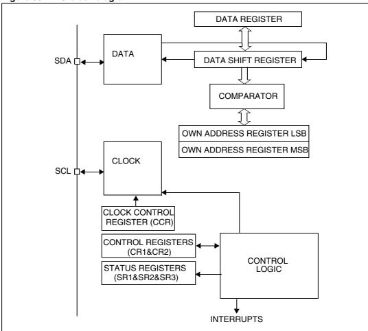
Figure 99. I<sup>2</sup>C block diagram
