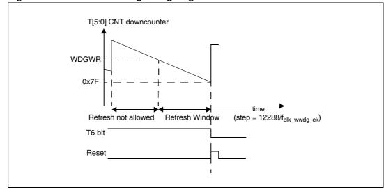
Figure 27. Window watchdog timing diagram
