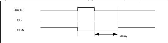
The deadtime delay is the same for each of the channels and is programmable with the DTG bits in the TIM1\_DTR register. Refer to *Section 17.7.31: Deadtime register (TIM1\_DTR) on page 208* for delay calculation.
