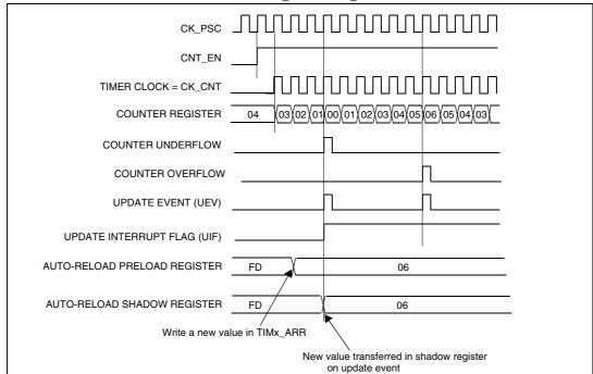
Figure 38. Counter timing diagram,  $f_{CK CNT} = f_{CK PSC}$ , TIM1\_ARR = 06h, ARPE = 1
