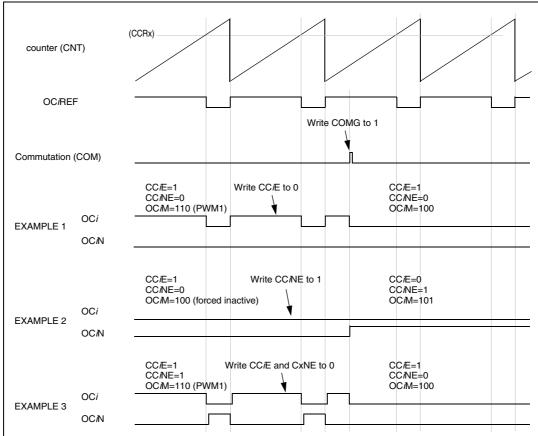
Figure 73. Six-step generation, COM example (OSSR = 1)
