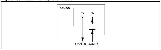
This mode is provided for self-test functions. To be independent of external events, the CAN Core ignores acknowledge errors (no dominant bit sampled in the acknowledge slot of a data / remote frame) in Loop Back Mode. In this mode, the beCAN performs an internal feedback from its Tx output to its Rx input. The actual value of the CANRX input pin is disregarded by the beCAN. The transmitted messages can be monitored on the CANTX pin.
