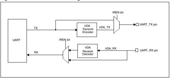
Figure 123. IrDA data modulation (3/16) - normal mode
