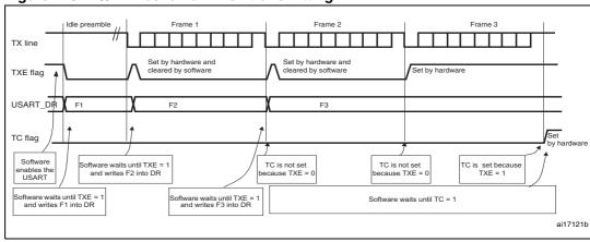
Figure 110. TC/TXE behavior when transmitting
