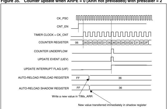
Figure 35. Counter update when ARPE = 0 (ARR not preloaded) with prescaler = 2
