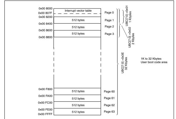
Figure 7. UBC area size definition on medium density STM8S
