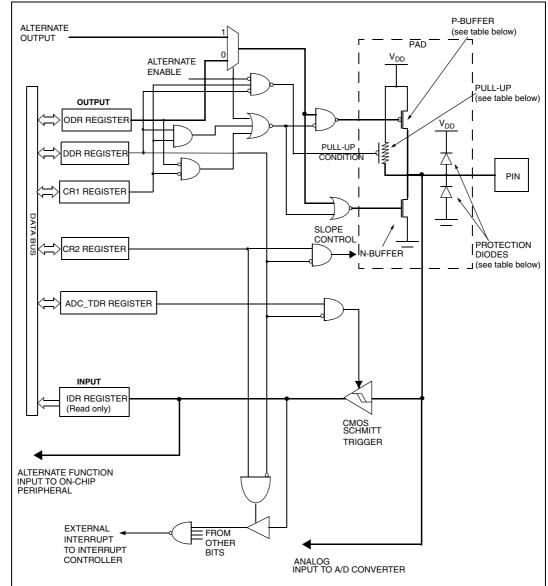
Figure 21. GPIO block diagram
