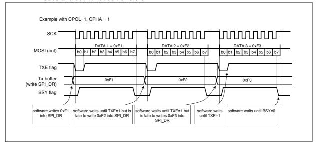
Figure 97. TXE/BSY behavior when transmitting (BDM = 0 and RXLONY = 0). Case of discontinuous transfers
