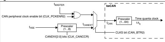
The frequency of the external clock f<sub>CANEXT</sub> must be less than that of the CPU clock (f<sub>CPU</sub>).
