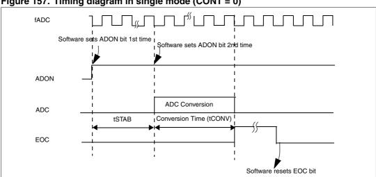
Figure 157. Timing diagram in single mode (CONT = 0)
