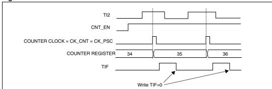
Figure 43. Control circuit in external clock mode 1
