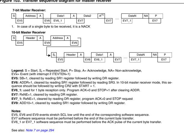
If the DR and shift registers are full, the next data reception (I<sup>2</sup>C clock generation for slave) is performed after the EV7 event is cleared. In this case, EV7 does not overlap with data reception.
