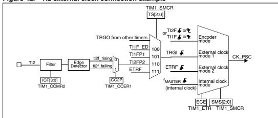
Figure 42. Tl2 external clock connection example
