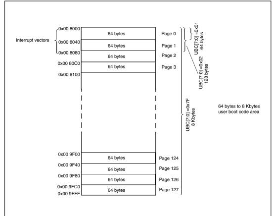
Figure 6. UBC area size definition on low density STM8S devices
