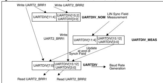
Figure 130. UARTDIV read / write operations when LDUM = 0
