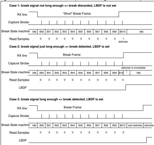
Figure 124. Break detection in LIN mode (11-bit break length - LBDL bit is set)
