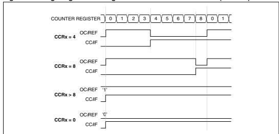
Figure 67. Edge-aligned counting mode PWM mode 1 waveforms (ARR = 8)
