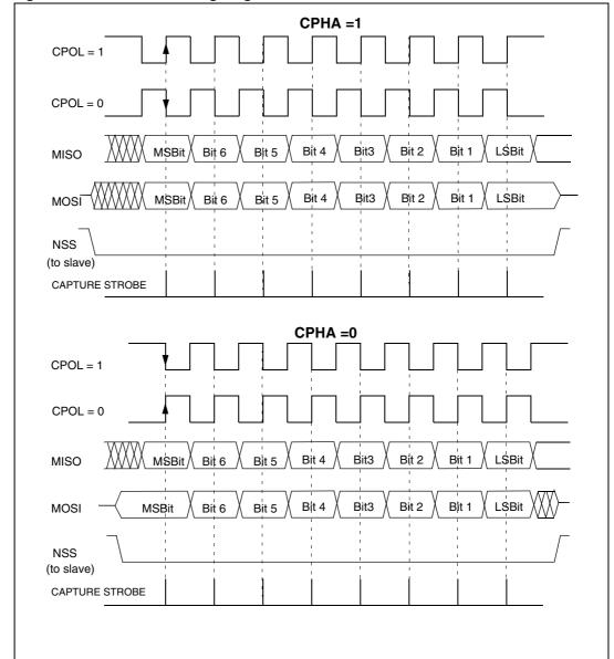
Figure 91. Data clock timing diagram
