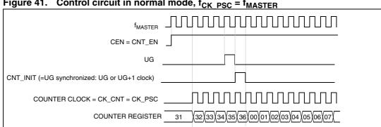
Figure 41. Control circuit in normal mode,  $f_{CK PSC} = f_{MASTER}$
