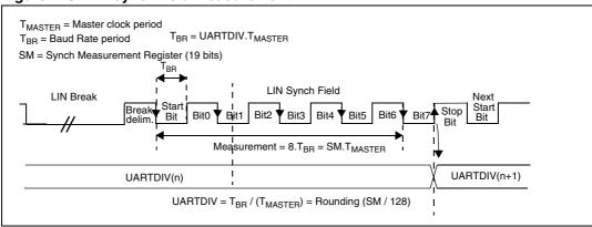
Figure 129. LIN synch field measurement
