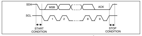
Acknowledge may be enabled or disabled by software. The I<sup>2</sup>C interface addresses (7-bit/ 10-bit and/or general call address) can be selected by software.
