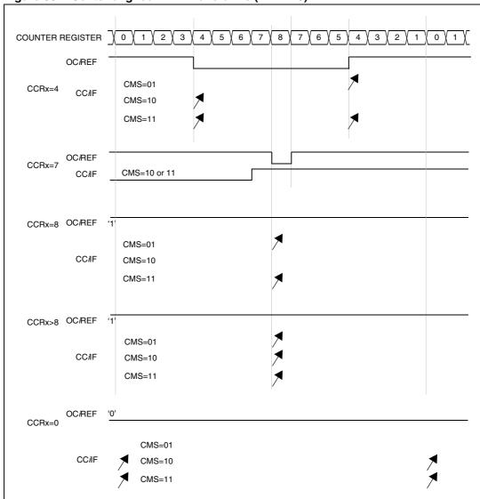
Figure 68. Center-aligned PWM waveforms (ARR = 8)
