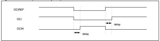
Figure 71. Deadtime waveforms with a delay greater than the negative pulse
