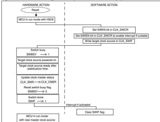
Figure 15. Clock switching flowchart (automatic mode example)
