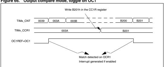
Figure 66. Output compare mode, toggle on OC1
