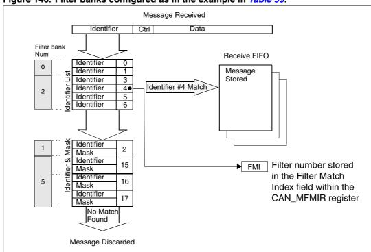
Figure 146. Filter banks configured as in the example in *Table 59*.
