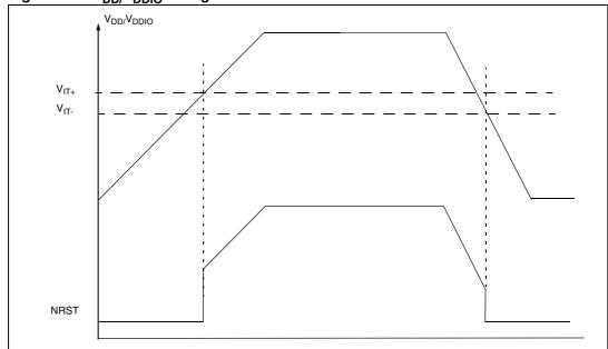
Figure 12. V<sub>DD/</sub>V<sub>DDIO</sub> voltage detection: POR/BOR threshold
