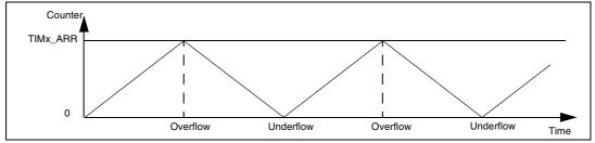
If the timer has a repetition counter (as in TIM1), the UEV is generated after up and down counting and repeated for the number of times programmed in the repetition counter register (TIM1\_RCR). Otherwise, the UEV is generated at each counter overflow and at each counter underflow.
