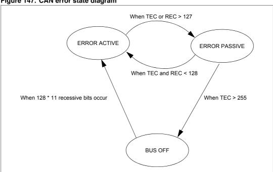
Figure 147. CAN error state diagram
