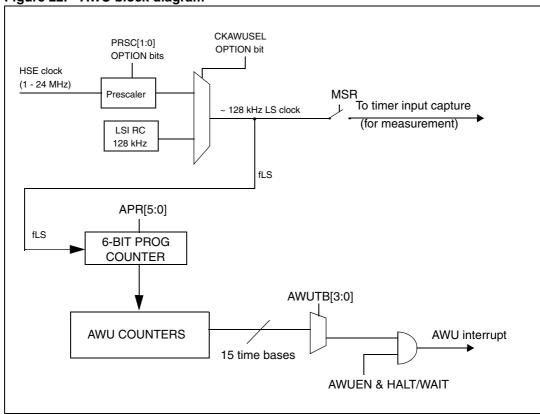
Note: The LS clock source is selected by programming the CKAWUSEL option bit as explained in the clock controller chapter.
