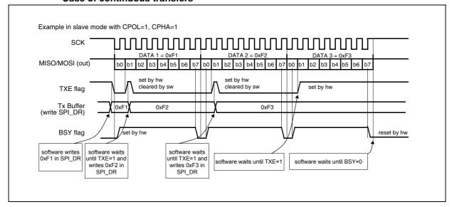
Figure 95. TXE/BSY in slave transmit-only mode (BDM = 0 and RXONLY = 0). Case of continuous transfers
