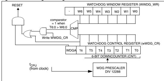
Figure 25. Watchdog block diagram
