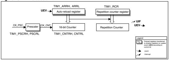
The 16-bit counter, the prescaler, the auto-reload register and the repetition counter register can be written or read by software.
