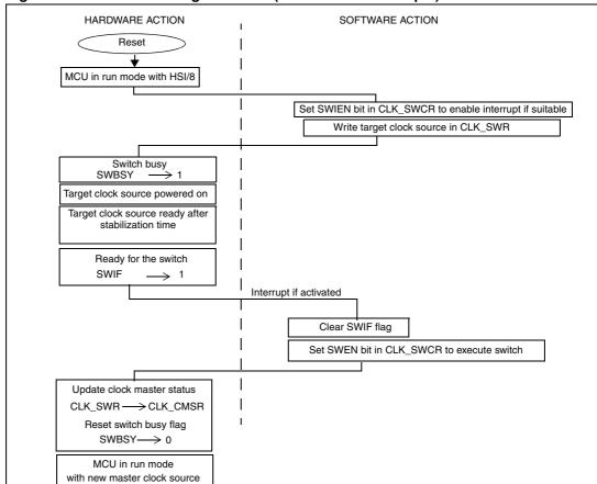
Figure 16. Clock switching flowchart (manual mode example)
