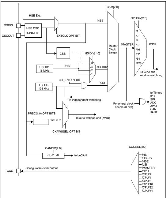
Legend: HSE = High speed external clock signal; HSI = High speed internal clock signal; LSI = Low Speed internal clock signal.
