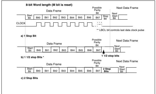
Figure 109. Configurable stop bits
