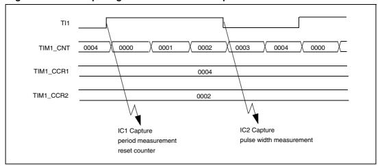
Figure 63. PWM input signal measurement example
