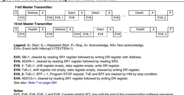
EV5, EV6, EV9, EV8\_1 and EV8\_2 events stretch SCL low until the end of the corresponding software sequence. EV8 software sequence must be performed before the end of the current byte transfer.
