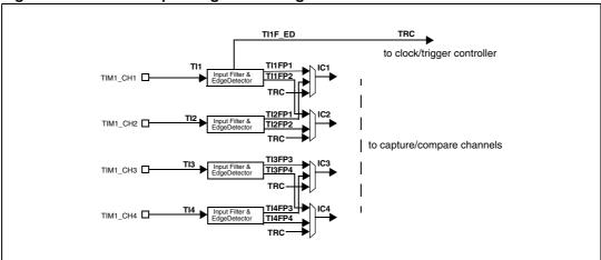
Figure 61 shows how the input stage samples the corresponding TIi input to generate a filtered signal TIiF. Then, an edge detector with polarity selection, generates a signal (TIiFPn) which can be used as trigger input by the clock/trigger controller or as the capture command. The signal is prescaled before entering the capture register (ICiPS).
