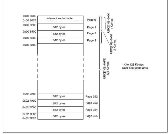
Figure 8. UBC area size definition on high density STM8S
