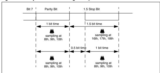
Figure 121. Parity error detection using 1.5 stop bits
