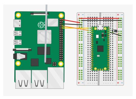
Whilst it is possible to connect the Raspberry Pi's 5V pin to the Raspberry Pi Pico VBUS pin, this is not recommended. Shorting the 5V rails together will mean that the Micro USB cannot be used. An exception is when using the Raspberry Pi Pico in USB host mode, in this case 5V must be connected to the VBUS pin.
