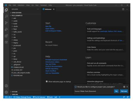
Go ahead and click on the "Build" button (with a cog wheel) in the blue bottom bar of the window. This will create the build directory and run CMake and build the examples project, including "Hello World".
