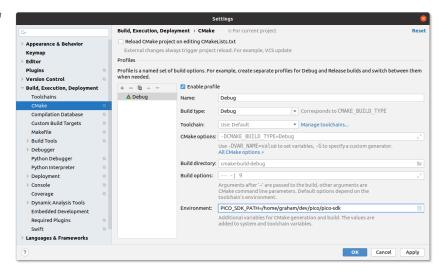
You can have as many CMake profiles as you like with different settings. You probably want to add a Release build by hitting the + button, and then filling in the PICO\_SDK\_PATH again, or by hitting the copy button two to the right, and fixing the name and settings (see Figure 33)
