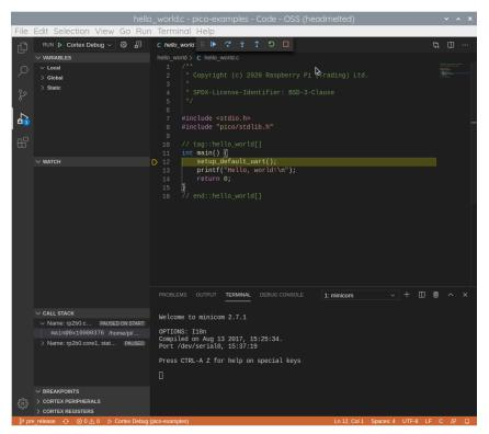
The code should now be loaded on to the Raspberry Pi Pico, and you should see the source code for "Hello USB" in the main right-hand (upper) pane of the window. The code will start to run and it will proceed to the first breakpoint — enabled by the runToMain directive in the launch.json file. Click on the small blue arrow (play button) at the top of this main source code window to Continue (F5) and start the code running.
