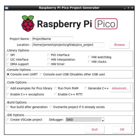
You can add specific features to your project by selecting them from the check boxes on the GUI. This will ensure the build system adds the appropriate code to the build, and also adds simple example code to the project showing how to use the feature.
