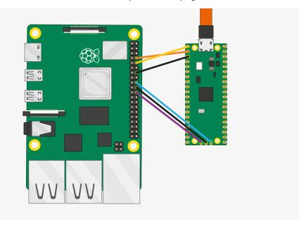
The default configuration is to have SWDIO on Pi GPIO 24, and SWCLK on GPIO 25 - and can be wired to a Raspberry Pi
