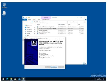
During installation you should tick the box to register the path to the Arm compiler as an environment variable in the Windows shell when prompted to do so.
