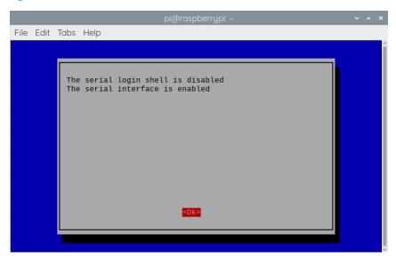
Leaving raspi-config you should choose "Yes" and reboot your Raspberry Pi to enable the serial port.
