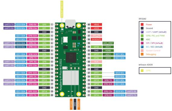
Raspberry Pi Pico W uses an on-board buck-boost SMPS which is able to generate the required 3.3V (to power RP2040 and external circuitry) from a wide range of input voltages (~1.8 to 5.5V). This allows significant flexibility in powering the unit from various sources, such as a single lithium-ion cell, or three AA cells in series. Battery chargers can also be very easily integrated with the Pico W powerchain.
