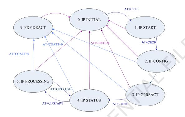
Figure3: APPTCP States Diagram for multi connection
