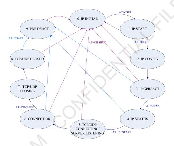
Figure2: APPTCP States Diagram for single connection
