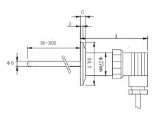
Figure 6-4 Hoop Connection No Display
