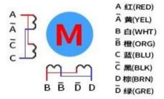
There are also motors which have non-standard line color, in this case, you can try to detect resistance of every two lines. If resistance is detected, set these two lines to one set.
