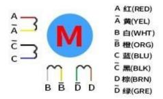
You can use two ways to connect four-phase eight lines stepper motor:
