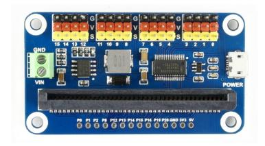
You can connect battery to the green socket VIN on the left for power supply, for VIM, voltage range 6V~12V. 5V regulator on board could output 3A (MAX) current.
