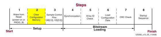
Figure 12-5: Clear Configuration Memory (Initialization)
