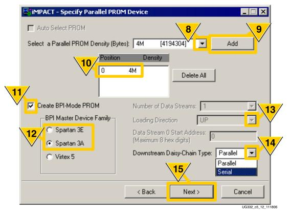
Figure 5-10: Select Parallel PROM Size and Configuration Style
