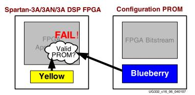
Figure 15-8: Authentication Fails Using an Unauthorized Copy
