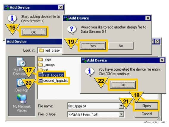
Figure 5-11: Select FPGA Bitstream Files
