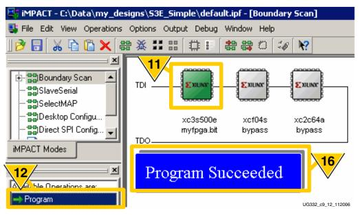
Figure 9-14: Double-Click Program to Configure FPGA via JTAG
