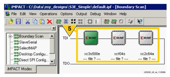
*Figure 9-9:* **iMPACT Automatically Detects Devices on the JTAG Chain**
