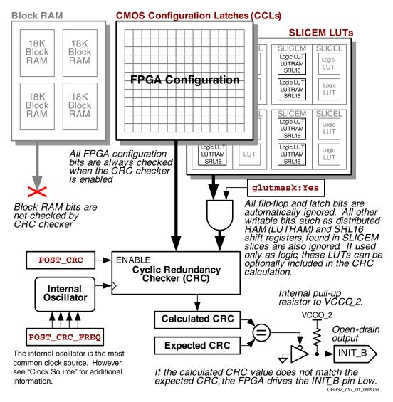
Figure 16-1: Conceptual Overview of Post-Configuration CRC Calculator
