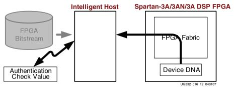
Figure 15-12: Host Reads Device DNA, Generates Authentication Value
