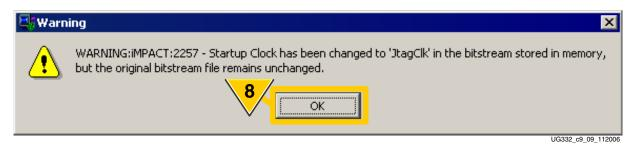
Figure 9-11: iMPACT Automatically Adjusts FPGA Startup Clock for JTAG Configuration
