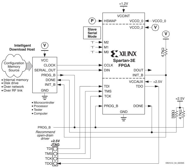
Figure 8-1: Slave Serial Configuration
