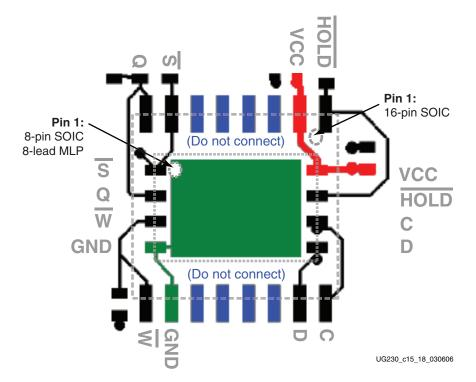
90°. The 16-pin SOIC package also has four pins at the center each side that do not connect on the board. These pins must be left unconnected, *i.e.* floating.
