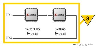
Figure 3-15: iMPACT Automatically Detects JTAG Chain
