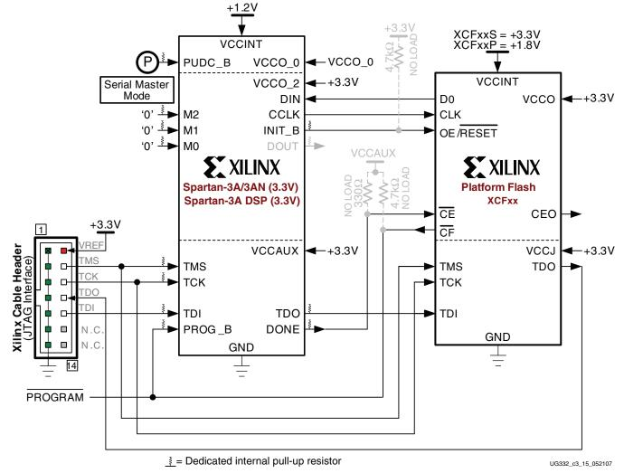
*Figure 3-2:* Master Serial Mode Using Platform Flash PROM (Extended Spartan-3A Family FPGA, V<sub>CCAUX</sub> = 3.3V)
