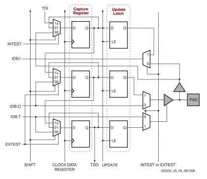
Figure 9-4: Boundary-Scan Logic per I/O Pin
