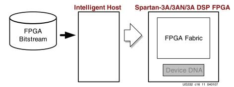
Figure 15-11: Intelligent Host Downloads a Spartan-3A Bitstream
