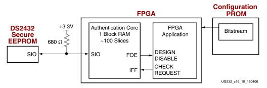
Figure 15-14: FPGA Authentication Using SHA-1 Secure EEPROM
