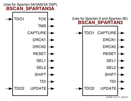
Figure 13-1: BSCAN Primitive for Extended Spartan-3A Family FPGAs
