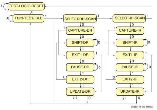
Figure 9-3: Test Access Port (TAP) State Machine
