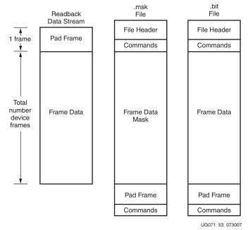
Figure 18-6: Comparing Readback Data Using the .msk and .bit Files
