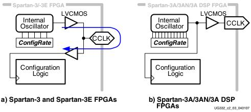
Figure 2-2: Differences between Spartan-3/3E and Extended Spartan-3A Family FPGAs for Master Configuration Modes
