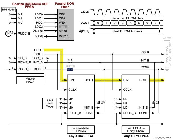
Figure 5-5: Serial Daisy Chains are Only Available for Extended Spartan-3A Family BPI Mode
