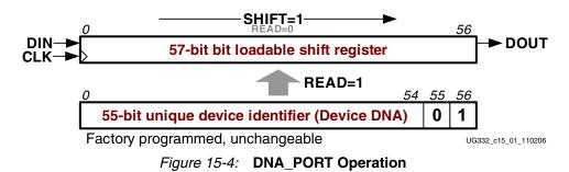
If both READ and SHIFT are Low, the output shift register holds its value and DOUT remains unchanged.
