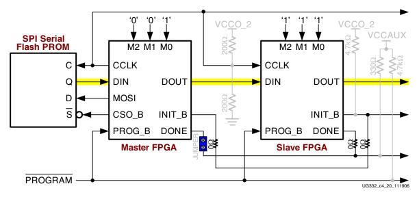
Figure 4-6: Daisy Chaining from SPI Flash Mode
