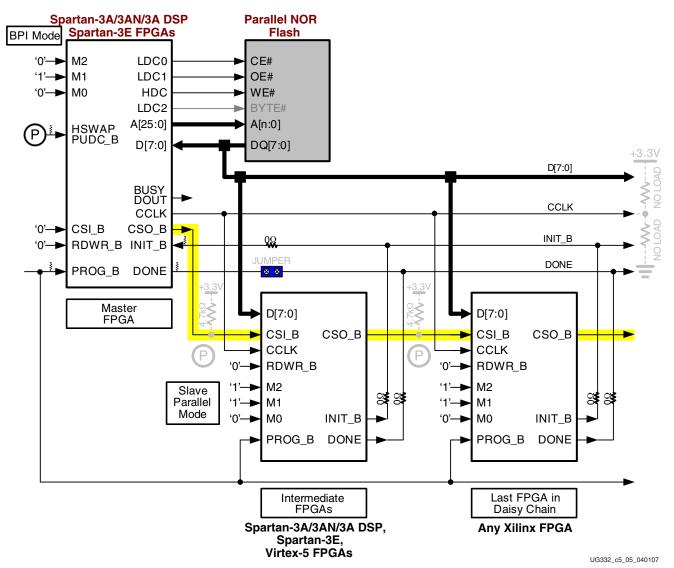
Figure 5-4: Parallel Daisy Chain using BPI Mode
