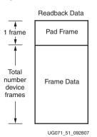
Figure 18-4: Readback Data Stream
