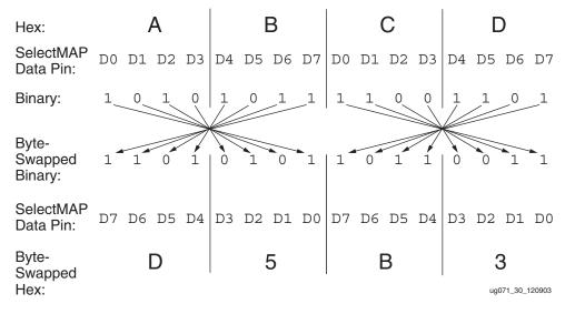
Figure 7-10: Byte Swapping Example
