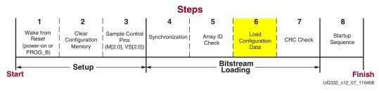
Figure 12-9: Load Configuration Data Frames
