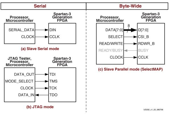
Figure 1-2: Spartan-3 Generation Downloaded (Slave) Configuration Modes
