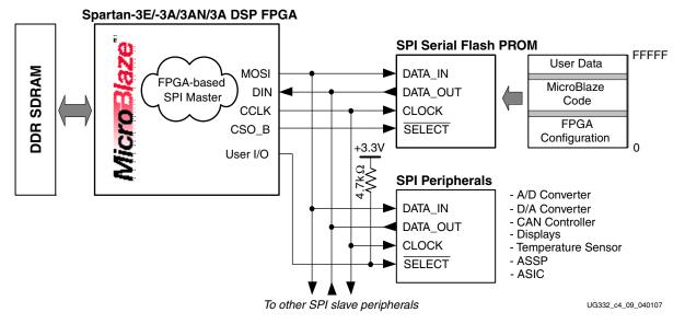
*Figure 4-5:* Using the SPI Flash Interface After Configuration
