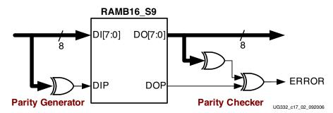
Figure 16-3: Checking Block RAM Contents Using Simple Parity
