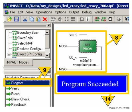
Figure 4-19: Directly Program Supported SPI Flash PROM.
