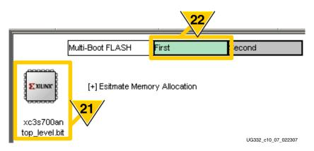
Figure 10-10: iMPACT View of the Spartan-3AN In-System Flash Memory
