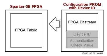
*Figure 15-9:* Spartan-3E FPGA Authentication Example using Commodity Flash PROM with Identifier
