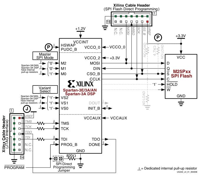
**Note:** Grayed out pull-up resistor on CSO\_B is only necessary when HSWAP/PUDC\_B is High (I/O Pull-Ups Not Enabled) Figure 4-1: SPI Flash Configuration Interface for M25P-compatible Devices
