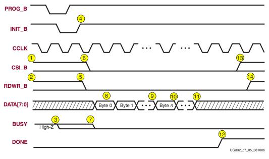
Figure 7-5: SelectMAP Continuous Data Loading
