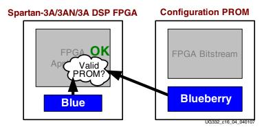
Figure 15-7: Extended Spartan-3A Family FPGA Authenticates the PROM Image Against Device DNA
