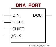
Figure 15-3: Extended Spartan-3A Family DNA\_PORT Design Primitive
