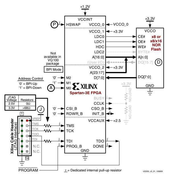
Figure 5-1: Spartan-3E FPGA Configured from Parallel NOR Flash
