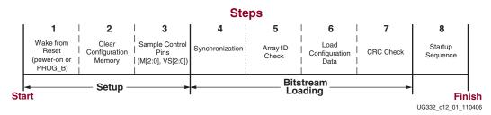
Figure 12-1: Spartan-3 Generation FPGA Configuration Process
