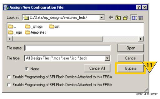
Figure 4-26: Bypass the Platform Flash PROM
