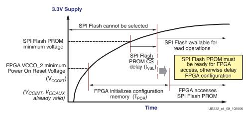
Figure 4-3: SPI Flash PROM/FPGA Power-On Timing if 3.3V Supply is Last in Power-On Sequence
