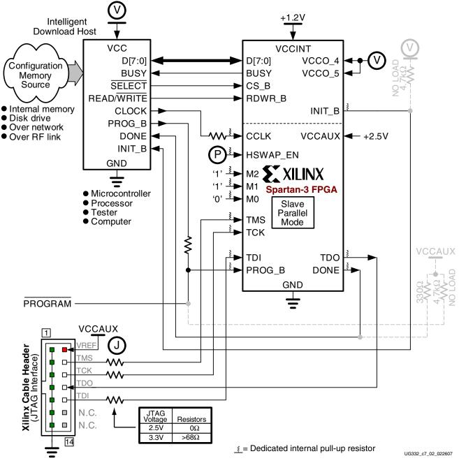
Figure 7-2: Slave Parallel Mode (Spartan-3 FPGAs)
