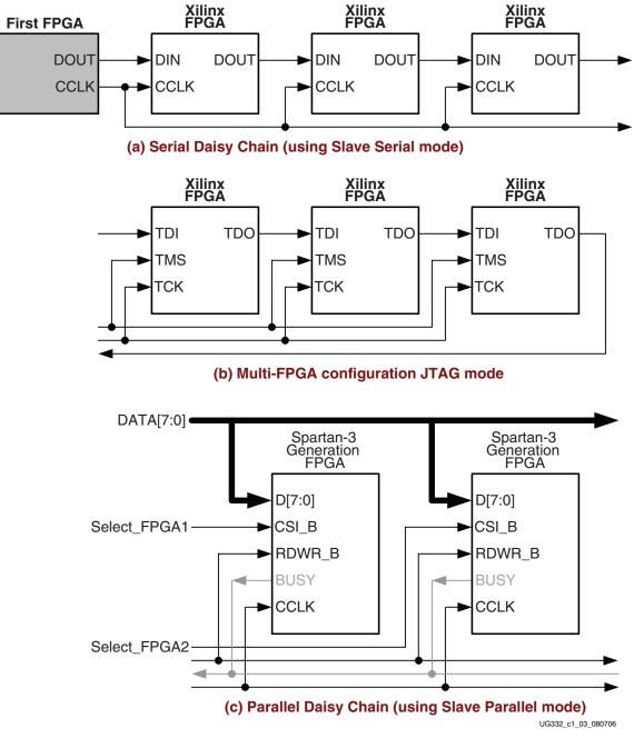
Figure 1-3: Spartan-3 Generation Configuration Daisy-Chain Options
