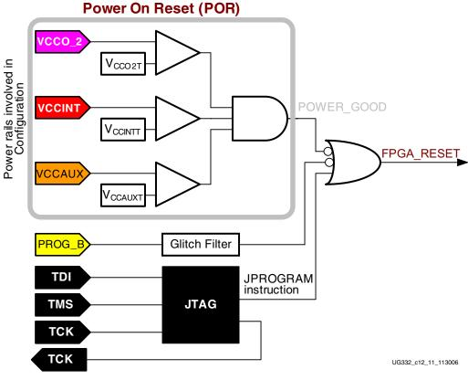
Figure 12-3: Extended Spartan-3A Family and Spartan-3E Reset Circuitry (Spartan-3 is similar)
