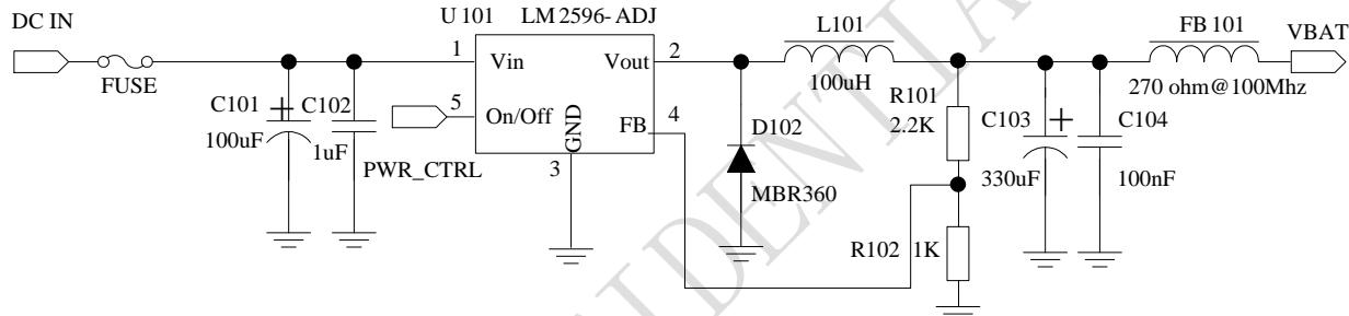
**Figure 9: Recommended circuits for switching power supply**
