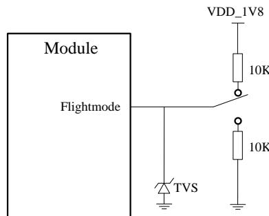
**Figure 27: Flight mode switch reference circuit**
