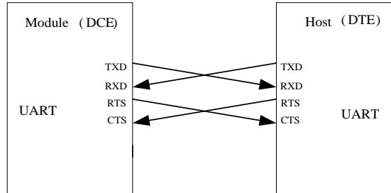
**Figure 14: Serial port connection diagram (full function mode)**
