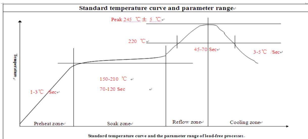
Figure 31: The ramp-soak-spike reflow profile of A7600E-H
