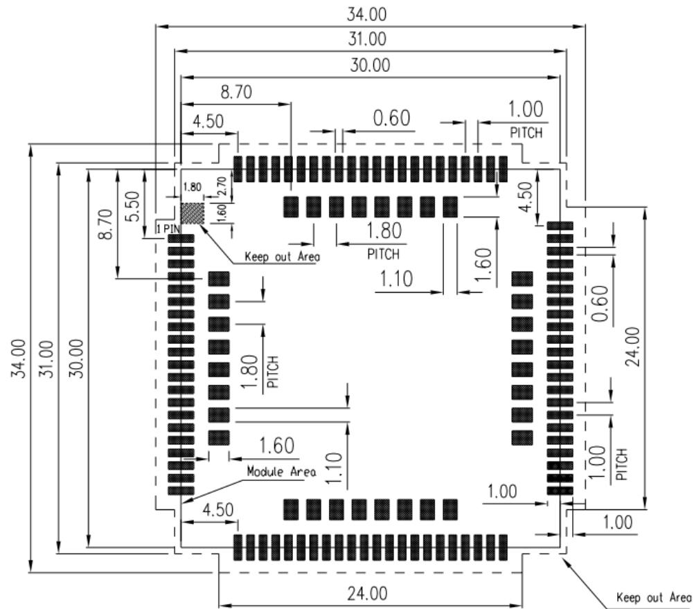
Figure 4: Recommend PCB footprint Dimension (Unit: mm)
