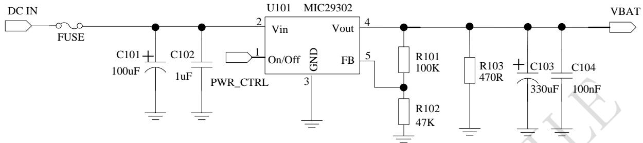
**Figure 8: Recommended circuit for linear power supply**
