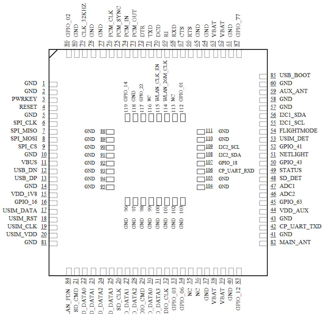
**Figure 2: Module pin diagram (Top view)**
