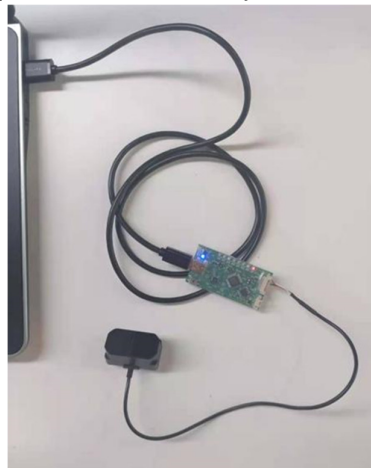
Fig.1 USB-UART converter connecting TFmini-Plus-IIC to PC
