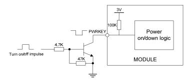
Figure 11: Powered on/down module using transistor
