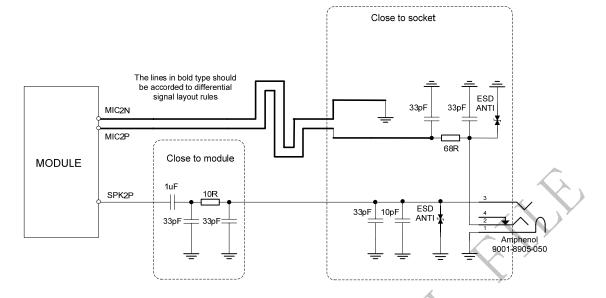
Figure 27: Earphone reference circuit
