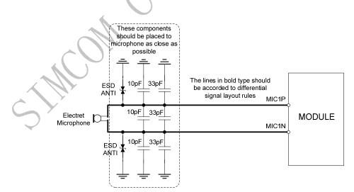
**Figure 26 : Microphone reference circuit**
