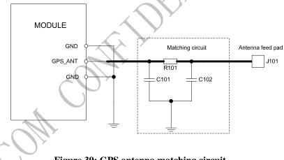
Figure 39: GPS antenna matching circuit
