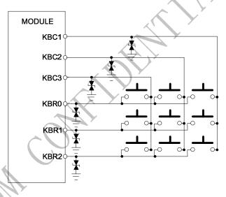
Figure 32: Reference circuit of the keypad interface
