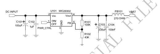
Figure 7: Reference circuit of the LDO power supply
