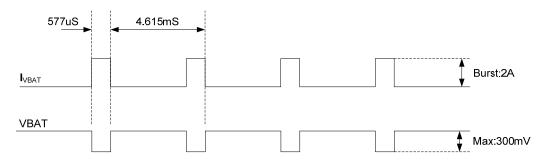
Figure 9: VBAT voltage drop during transmit burst
