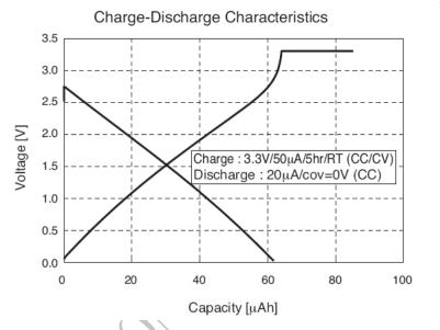
Figure 20: Seiko XH414H-IV01E charge-discharge characteristic
