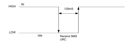
Figure 35: RI behaviour of URC or receive SMS
