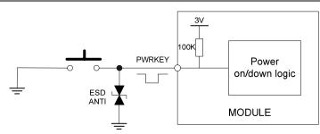
Figure 12: Powered on/down module using button
