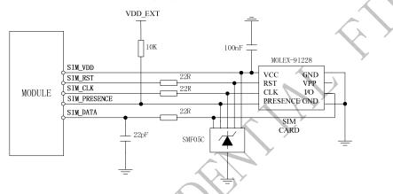
Figure 28: Reference circuit of the 8-pin SIM card holder
