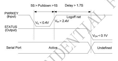
Figure 14: Timing of power down SIM908 by PWRKEY
