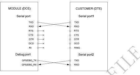
Figure 22: Connection of RXD and TXD only
