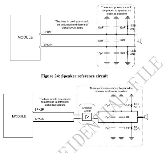
Figure 25: Speaker with amplifier reference circuit
