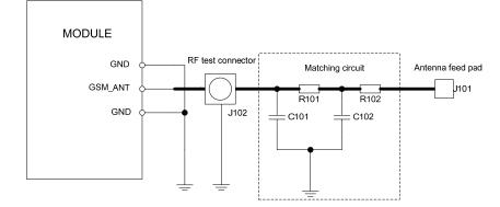
Figure 38: GSM antenna matching circuit
