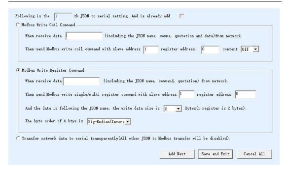
Figure 26 Sending JSON to Modbus
