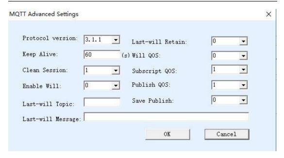
Figure 34 MQTT advanced parameter configuration
