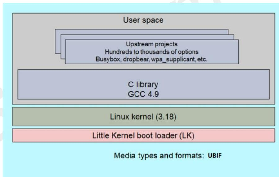
The SIM7600 is based on the ARM Cotex-A7 1.3GHz CPU and runs the Linux operating system. The kernel version is 3.18.20. The file system uses the UBIFS file system. The Linux-managed ubi file system contains three logical partitions:
