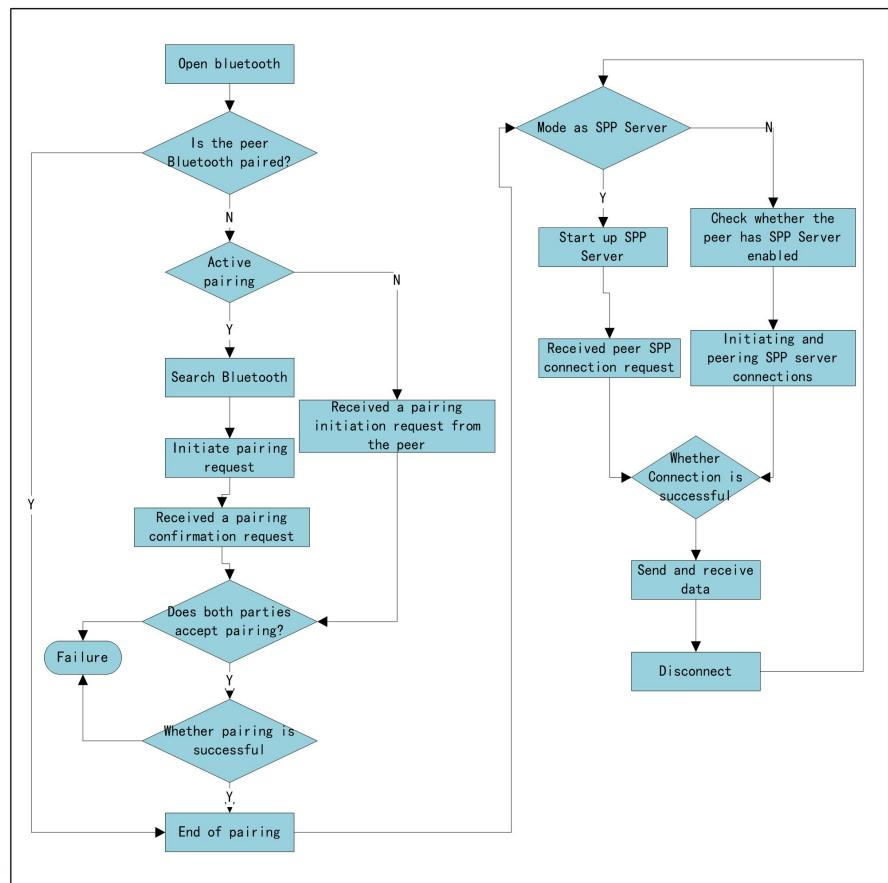
Bluetooth SPP pairing and SPP data transceiver flow chart
