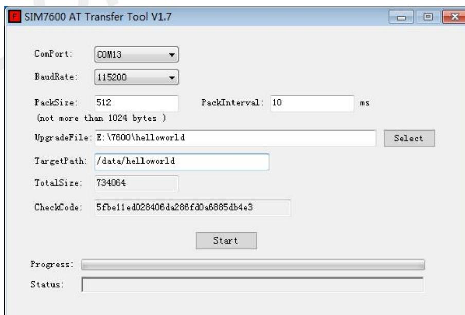
The basic principle of this tool is that the customer selects his own compiled application file and then selects Down File. The tool will place this program in the module /data and /usr/bin directory and rename it 'helloworld', and then automatically modify it to executable permissions. The next time the module is booted, it will automatically check if there is helloworld under data. If so, it will automatically execute and complete the client's program startup.
