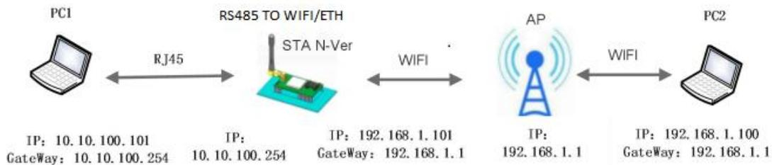
Figure Wired and Wireless Networking Application (Routing)
