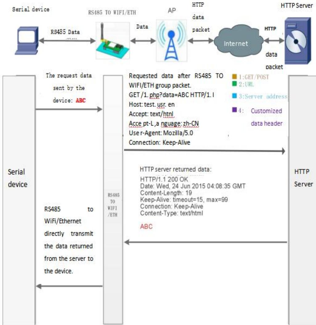
Figure HTTPDClient functional block diagram
