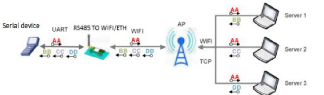
Figure multi-TCP link data transmission diagram
