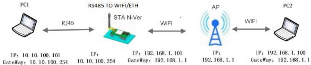
Figure Wired and Wireless Networking Application (Routing)
