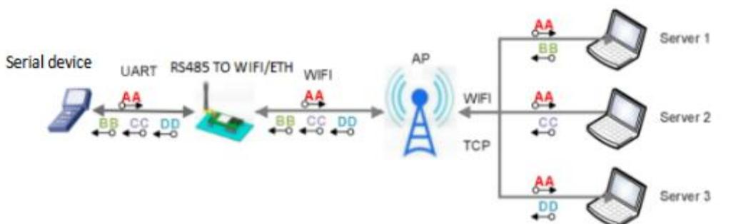
Figure multi-TCP link data transmission diagram
