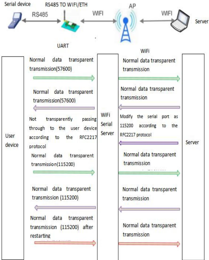
Figure RFC2217 automatic baud rate
