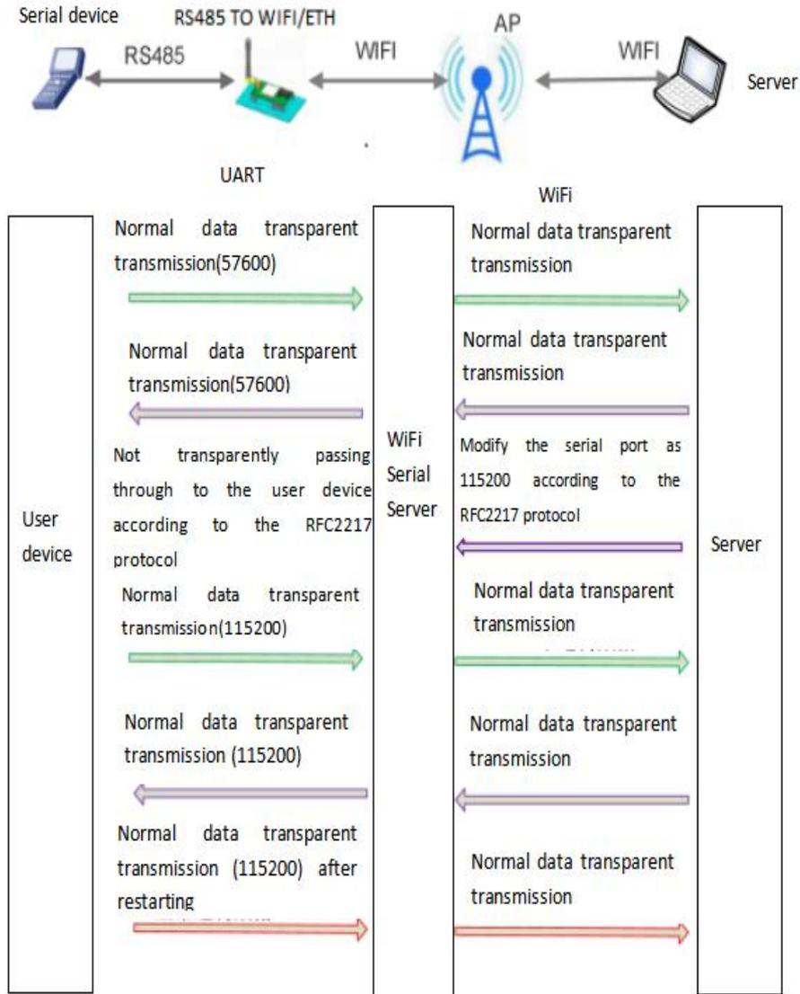
Figure RFC2217 automatic baud rate
