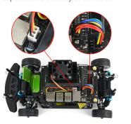
7. Mount camera on its holder by nylon screws. Note that the Acrylic board should be put between camera and the metal holder to avoid shorting. Finally, assemble the antenna.
