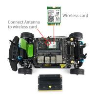
6. Replace Jetson Nano. Assemble cooling fan by its own screws. Connect the wires to the fan interface. Connect the Jestson Nano Developer Kit to JetRacer Expansion board by 6PIN wires.
