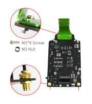
3. Fix JetRacer Pro Expansion board on chassis.
