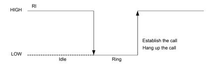
Figure 26: UART1\_RI behaviour of voice calling as a receiver
