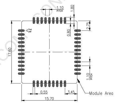
Figure 5: Recommended SMT stencil footprint outline (Unit: mm)
