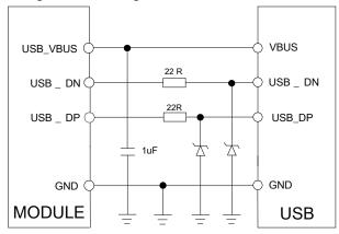
Figure 24: USB reference circuit
