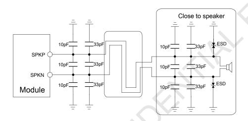
Figure 29: Speaker reference circuit
