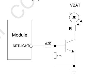
Figure 35: Reference circuit of NETLIGHT
