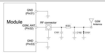
Figure 37: GSM antenna matching circuit
