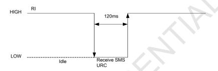
Figure 27: UART1\_RI behaviour of URC or receive SMS
