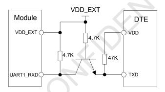
Figure 23: RX level matching circuit
