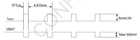
Figure 9: VBAT voltage drop during transmit burst
