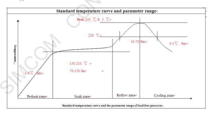
Figure 42: Typical solder reflow profile of lead-free processes
