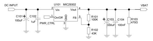
Figure 7: Reference circuit of the LDO power supply
