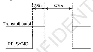
Figure 36: RF SYNC signal during transmit burst
