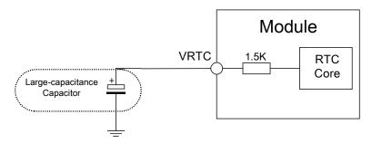
Figure 16: RTC supply from capacitor
