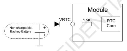
Figure 17: RTC supply from non-chargeable battery
