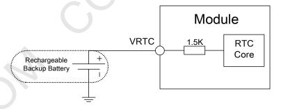
Figure 18: RTC supply from rechargeable battery
