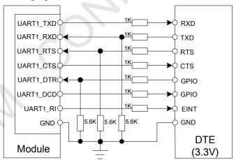
Figure 20: Resistor matching circuit
