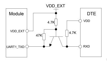
Figure 22: TX level matching circuit
