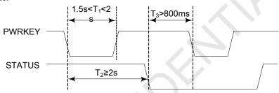
Figure 15: Timing of restart SIM800C
