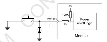
Figure 12: Powered on/down module using button
