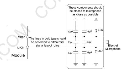
Figure 30: Microphone reference circuit
