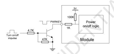
Figure 11: Powered on/down module using transistor
