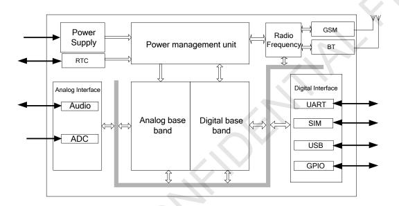
Figure 1: SIM800C functional diagram
