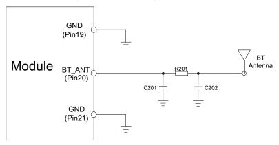
Figure 39: Bluetooth antenna matching circuit
