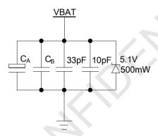
Figure 6: Reference circuit of the VBAT input
