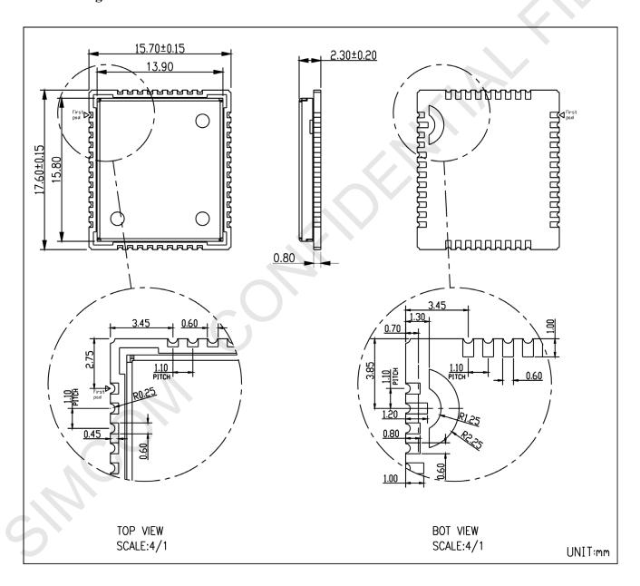
Figure 3: Dimensions of SIM800C (Unit: mm)
