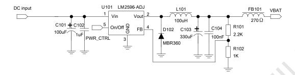
Figure 8: Reference circuit of the DC-DC power supply
