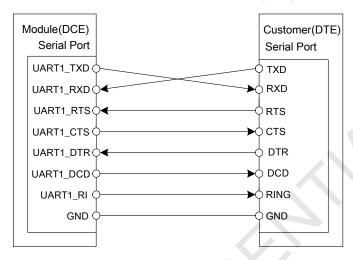
Figure 19: Connection of the serial interfaces
