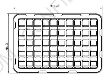
Figure 44: Module tray drawing
