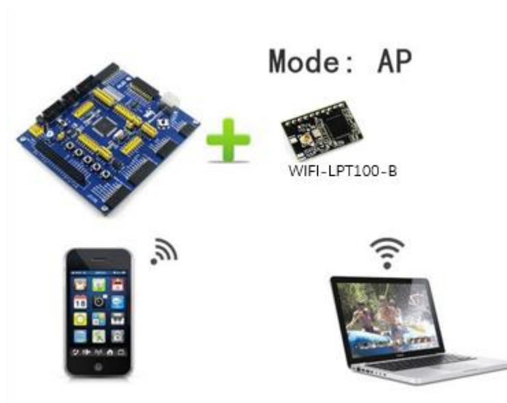
Figure 17 WIFI-LPT100-B AP Networking Structure
