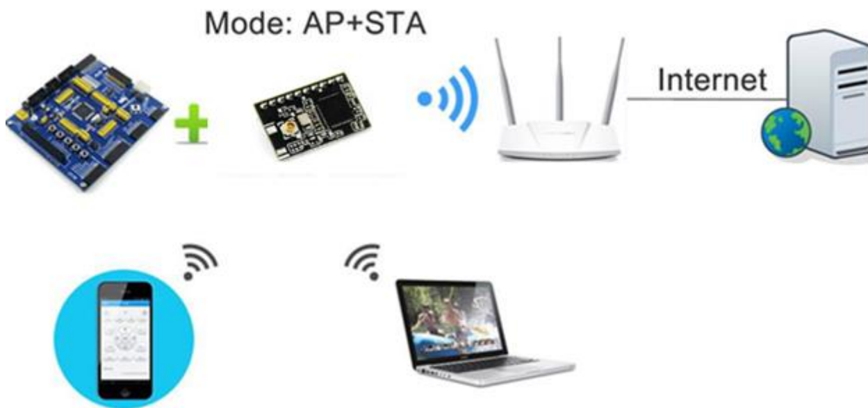
Figure 18 WIFI-LPT100-B AP+STA Networking Structure
