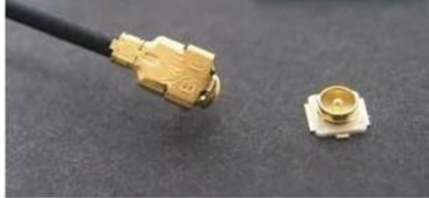
Figure 13 WIFI-LPT100-B I-PEX Connector
