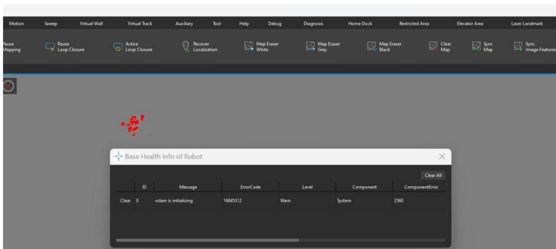
The equipment needs to remain stationary for 3 to 4 seconds during initial operation to complete system initialization. The specific operation recommendations are as follows:
