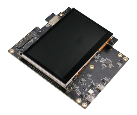
Default settings: \* BSP example `display\_lvgl\_demos` \* LCD: 4.3" 800x480 \* Interface: RGB \* LVGL buffer size: 800 x 100 \* LVGL double buffer: N0 \* Optimization: Debug \* CPU frequency: 160 MHz \* Flash frequency: 80 MHz \* Flash frequency: 80 MHz \* Flash mode: DI0 \* LVGL display refresh period: 30 ms
