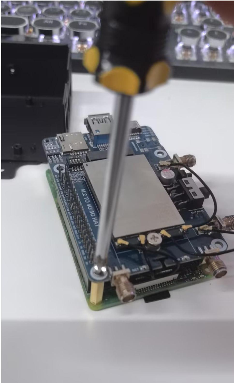
**Assemble the 5G HAT and Raspberry Pi, and then put the whole thing on the bottom shell**
