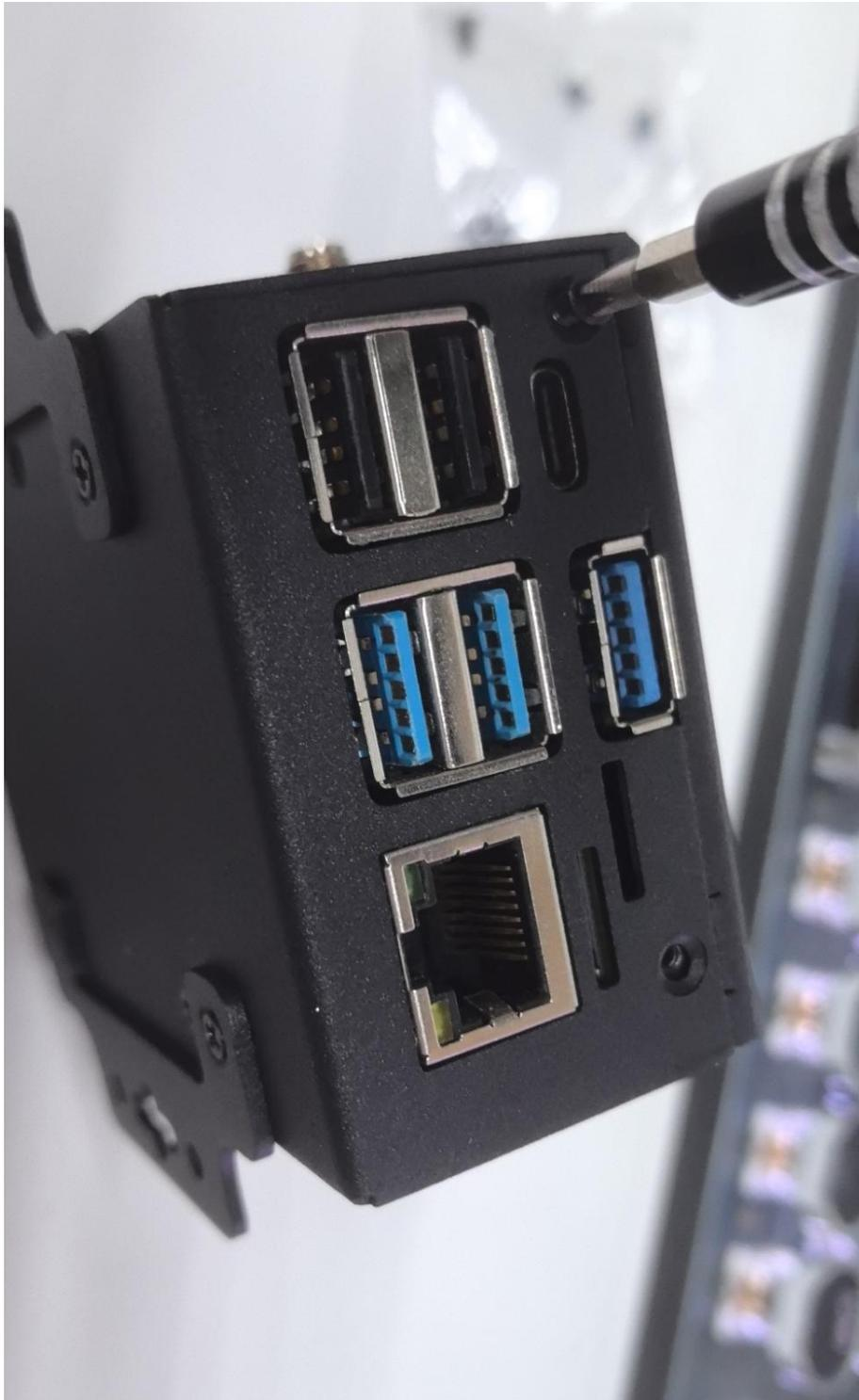
**Install the wall-mounted ears or rail buckles on the shell**
