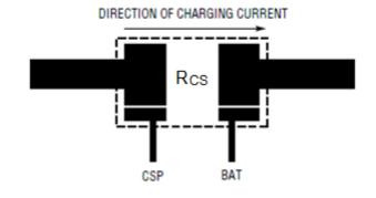
Figure 5 Kelvin Sensing of Charge Current
