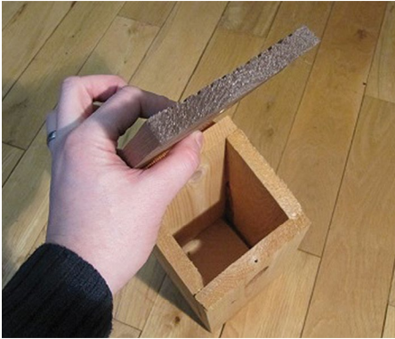
Figure 3 Pinch the lid and then use a pen to mark a cross where your thumb is
