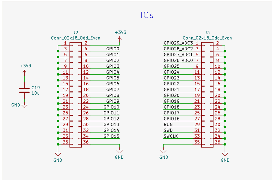
Figure 12. Schematic section showing the 2.54mm I/O headers of the QFN60 version
